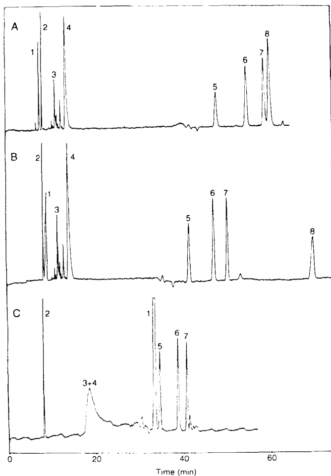
Figure 6. Electropherograms of polymyxins B and six test substances obtained at (A) pH 2.5, (B) pH 4.0, (C) pH 6.0 and (D) pH 8.0. Capillary, 75 \mu\text{m} I.D.; buffer, 25 mM PAPS in 0.2 M sodium phosphate pH 2.5, 4.0, 6.0 or 8.0 – water (1:1, v/v); voltage, 15 kV at pH 2.5, 4.0 and 6.0 and 10 kV at pH 8.0; hydrostatic injection, 2 s. (1) Aniline, (2) \beta -phenylethylamine, (3) polymyxin B 2 , (4) polymyxin B 1 , (5) benzyl alcohol, (6) phenol, (7) p-cresol, (8) benzoic acid.
